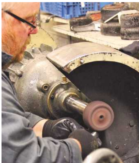
▲ All the bright work is polished by hand on buffing wheels
